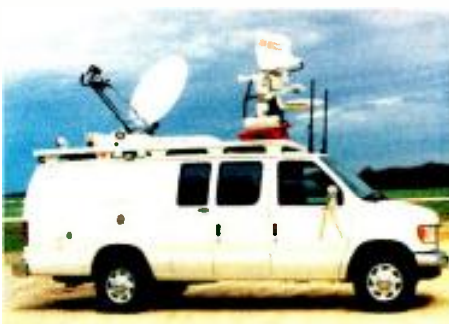
TEC has developed a kit to retrofit its ENG trucks for digital SNG capability.
